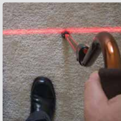
Left: Example of a laser cane to prompt bigger steps.
